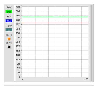
As long as the current measurement value **RAW** (green line) lies above the switching threshold (red line), the output **OUT0** has +24V (signal is OK). This is visualised by the **OUT0** LED.
